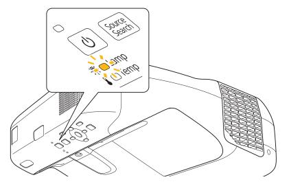
• The projected image gets darker or starts to deteriorate.
