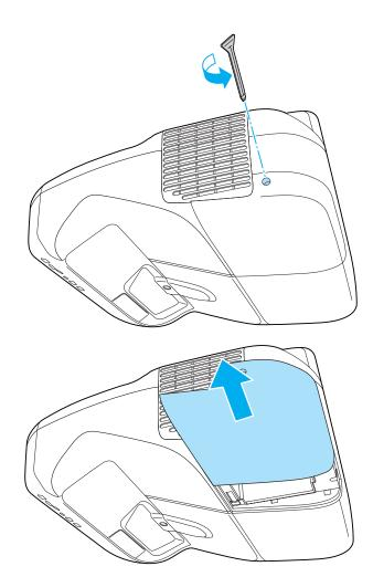
3 Loosen the two lamp fixing screws.
