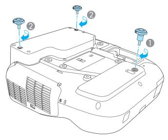
• Insert the foot with the spacer into the front foot fixing point.
