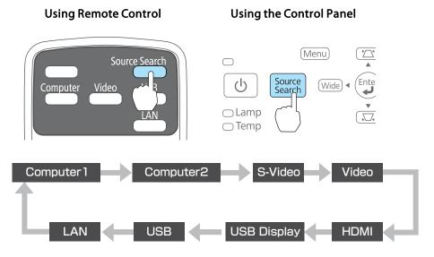
When two or more image sources are connected, press the [Source Search] button until the target image is projected.
